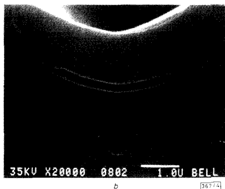
Fig. 4 a SEM photograph showing the growth of a buried crescent InP/GaInAsP/InP multilayer structure over a V-groove by CBE b A magnified view of the buried crescent structure
